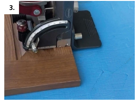
3. Run 14mm deep P-System slots on back of drawer face
