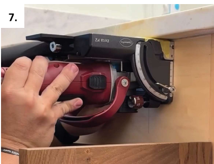
7. Run 10mm deep P-System slots into false front backer, corresponding to those on drawer face
