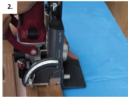
2. Use stop square to create an outside reference fence
