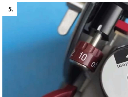
5. Set Zeta P2 to the 10mm depth setting for the Tenso P-14 connectors on the false front backer
