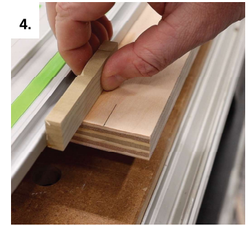
4. Using a piece of scrap wood, cut spacers to match your reveal
