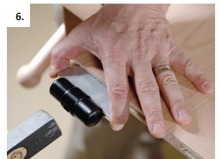
6. Install female halves into shelf edges with Divario install tool
