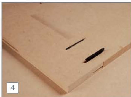
4 ... or you can butt joint at 90° for frame making or for mitered sections
