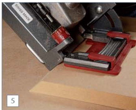
5 To make the mitered version, butt two pieces together. Set up your biscuit joiner to 45° and cut a slot across both inside edges on the mitered faces using the number 20 setting
