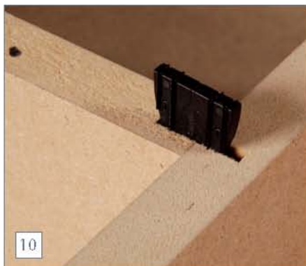
10 You can use the Fixo for T-joints too
