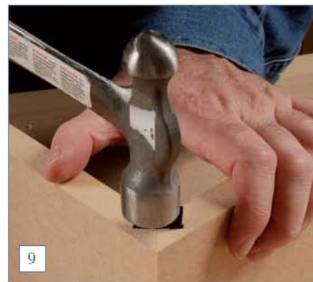
9 Tap in the fixing on one side, turn over and tap in the fixing on the other. These are dry but apply some glue as well and the result is a very strong joint
