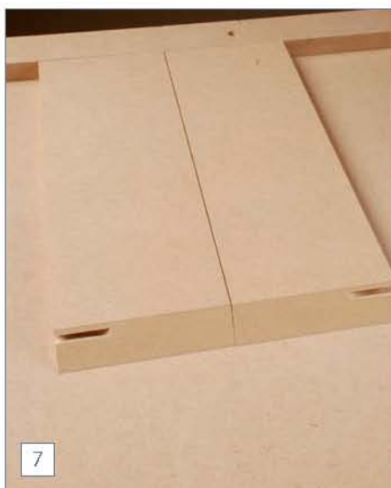
7 Turn the slotted edges to the outside and repeat the process – note the use of a support board. This is like a large bench hook and acts as a reference surface & holding device
