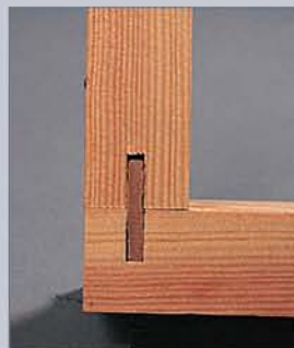
Butt corner joints can be achieved in seconds with a biscuit or two...
