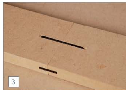
3 The other type of fixing will lock short lengths together on the side and on the top face...
